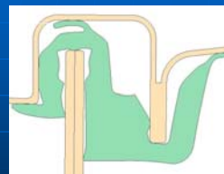
Jyco's Cross-section of Rear Door Sail Mold
